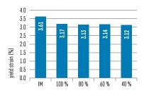
yield strain - a material characteristic which indicates the elongation of the material at the point of plastic deformation
